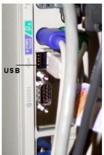
Attach the other end of the connector cable to the USB port on the EdgePort. EdgePort/4
